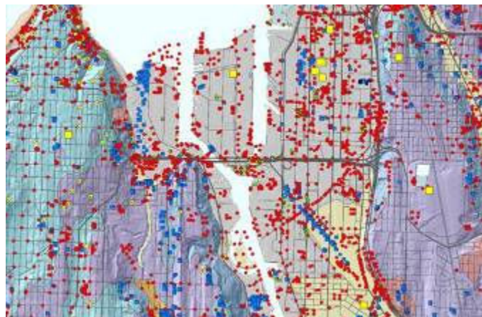
New GeoMapNW geologic map of Seattle SoDo area showing distribution of available subsurface data (red and blue dots)
